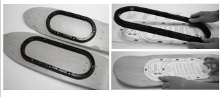
**Step 1:** Decide which rail size you want. The 4" extension pieces can always be added later. Make sure the rail fits the exact hole placement on the template. Cut out the template and tape it to the board top. You can place the rail in the center or closer to the end of the board. The rail allows for slight bending to conform to a bent board.
