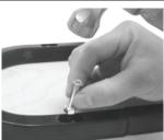
**Step 5:** Place the nut inside the recessed slot on the bottom of the rail. The nut fits snug and should be placed over the bolt. It is easier to turn the nut 90°, push it in and then turn it level. A second option is to reverse thread a nut and bolt, tap it in place then remove the bolt.
